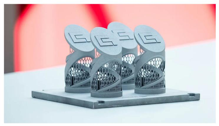
Additive manufacturing processes can be applied to fabricate topology-optimized parts. Image courtesy Grenzebach
