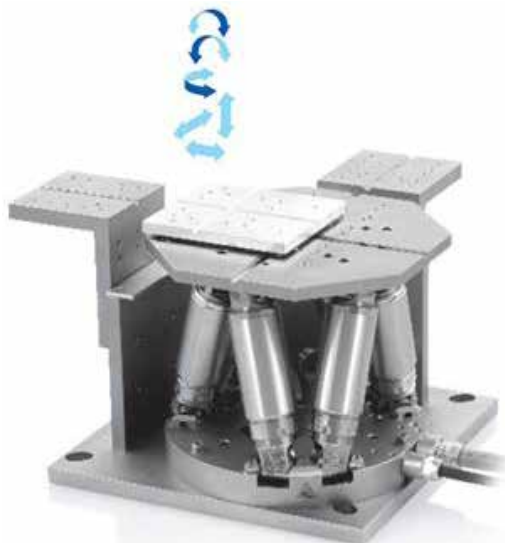
■ Figure 4: This micro-hexapod 6-D aligner offers extreme flexibility along with very high dynamics, stiffness and stability due to its parallel kinematics design with extremely low moving masses. Another advantage of the hexapod design is the randomized pivot point, programmable with one single command.
