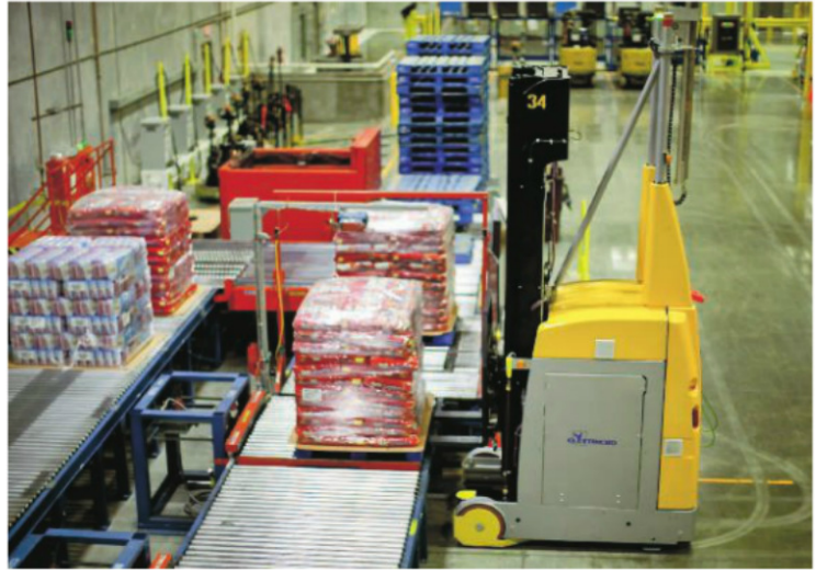
LGVs connect islands of automation between robotic case palletizing, stretch-wrapping, pallet labeling and transport to the warehouse.
