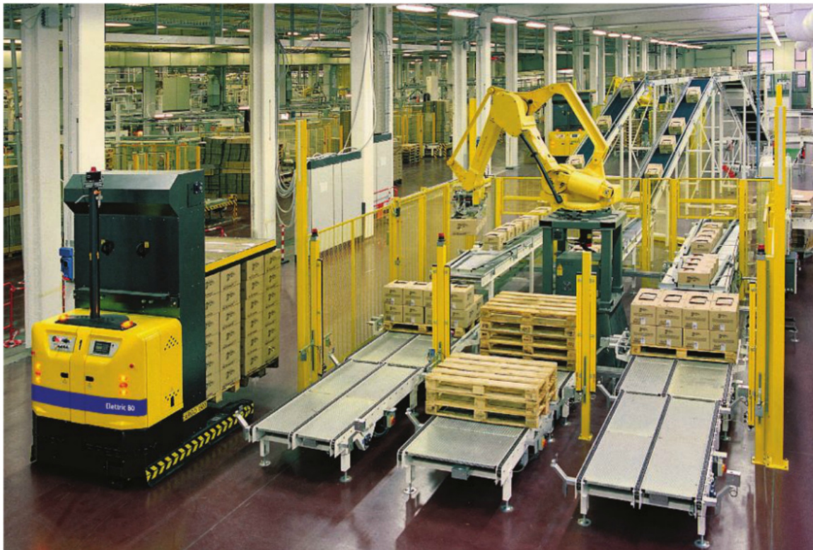
An end-of-line robotic palletizing station interfaced with LGVs.
