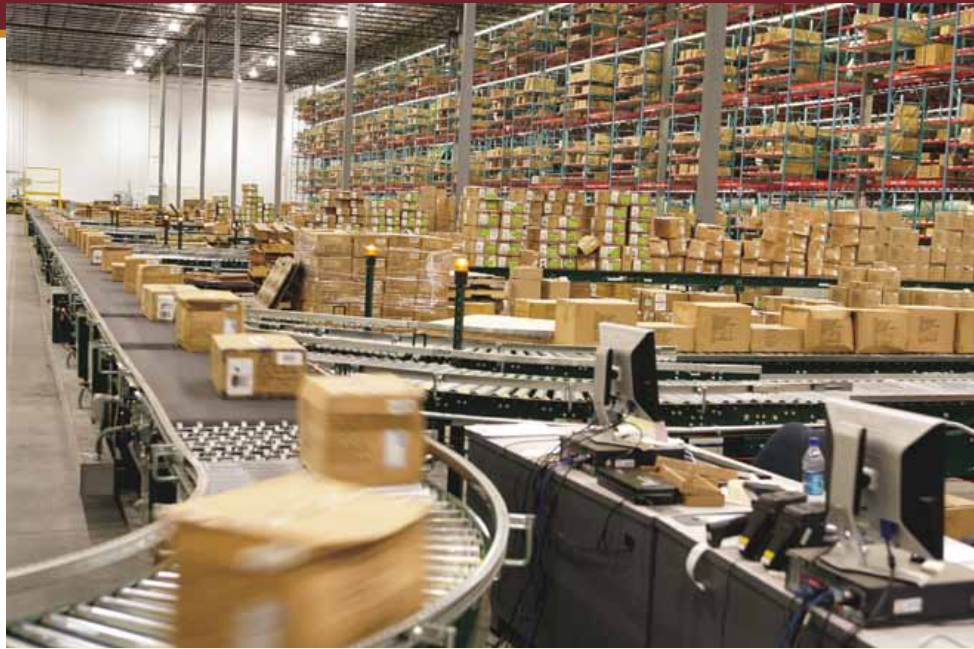
Individual cartons are automatically delivered for putaway in one of the high bay storage areas.
