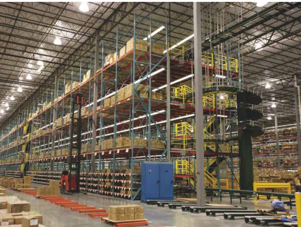
A high reach lift truck is used to put away pallets in one of the high bay storage areas.
