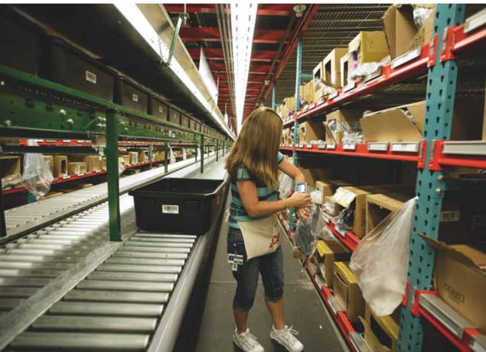
Piece picking is directed by pick-to-light, voice, or, in this case, to an associate using a ring scanner that enables hands-free picking.
