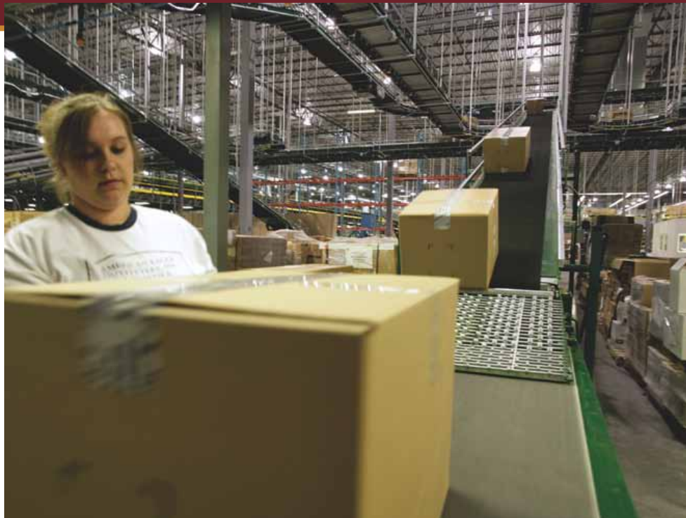
Some cartons are automatically crossdocked from the receiving dock to the shipping dock for store replenishment.
