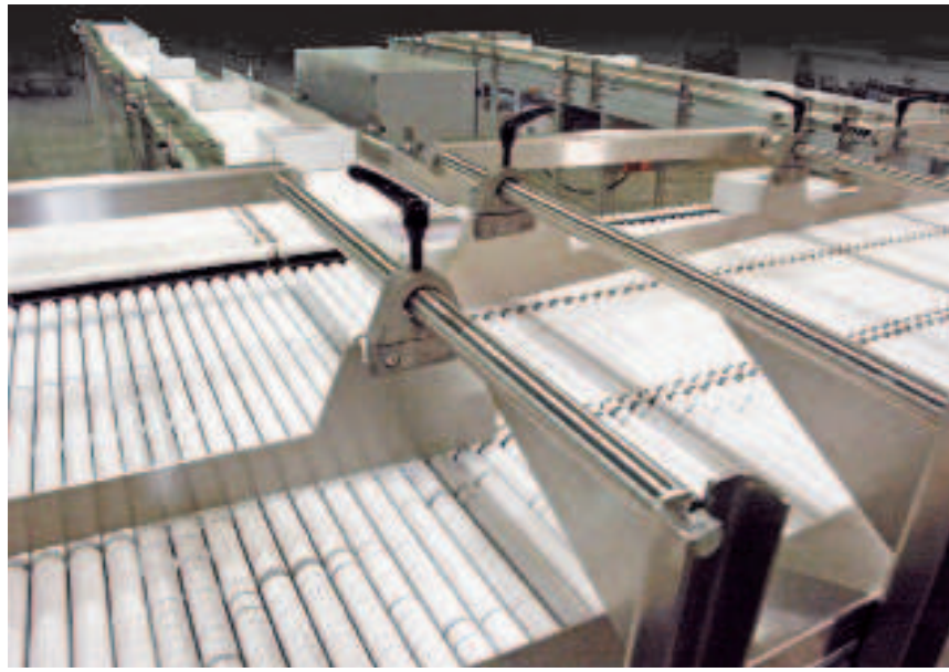
The Slip-Torque low back-pressure accumulation system stages cheesecake cartons for entry into the case packer.
