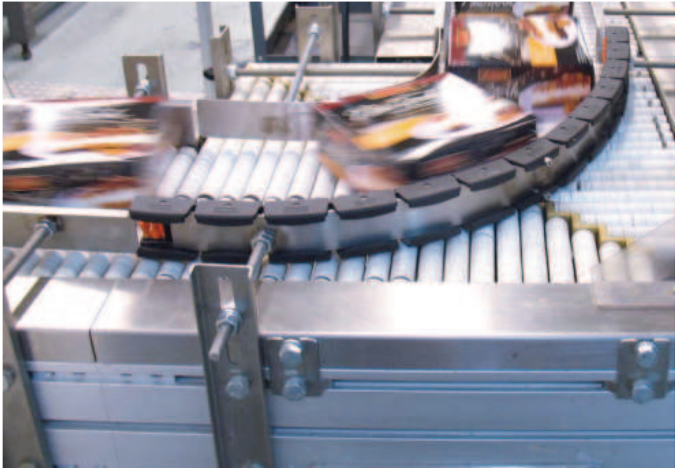
Motorized rollers can modulate the speed of different sections of the conveyor using a central-control HMI.
