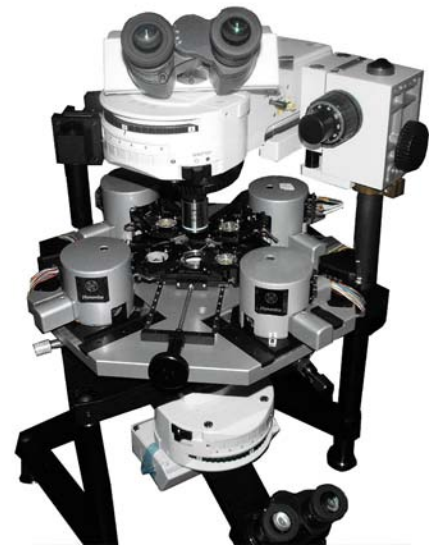
Minus K - Nanonics MultiView 4000 MultiProbe system for scanning probe microscopy permits full integration with optical techniques such as Raman using negative-stiffness vibration isolation.
