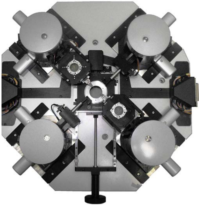
The MicroView4000 platform from Nanonics Imaging is the basis for AFM-Raman integration.
