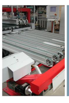
The first piece of Grenzebach equipment to exclusively utilize this advanced automation technology is the company's new High-Speed Stacker. Designed to increase glass manufacturer's efficiency and flexibility, it was developed for stacking small glass formats with high cycle times, and is currently the only device which can stack glass sheets in less than a one-second cycle.
