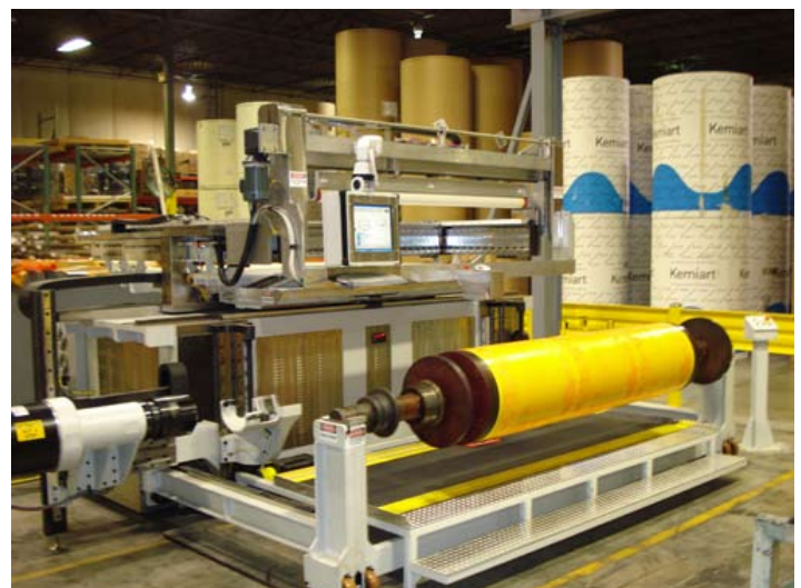
Mounter with cylinder loading mechanism and laser gauge for checking cylinder quality before mounting - Leader Engineering
