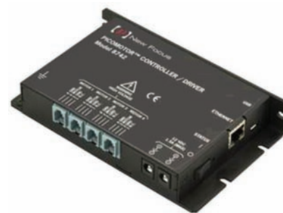
New Focus offers piezo-based nanopositioners including the Picomotor and Agilis from parent company Newport. Courtesy of New Focus.
