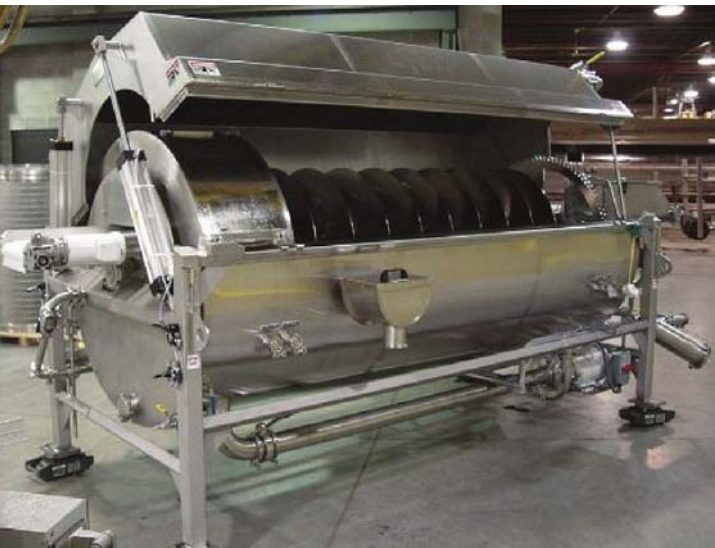
Above Clean-Flow provides quick-cleaning for changeovers and adds a water injection feature for added agitation to keep the rice in uniform suspension while moving through the process.
