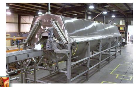
course, deeper loads require more time to bring the entire load, including the center of mass in the machine, to processing temperature, which necessitated longer blanch times; consequently, the beans on the outside of the mass were overcooked. Deeper loads also can cause the top portion of the relatively static load to ride out of the water, causing those beans to be undercooked.
