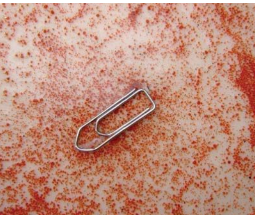
The DEMON process utilizes a consortium of anammox, which is often recognized by an intensely red color, as shown above.
