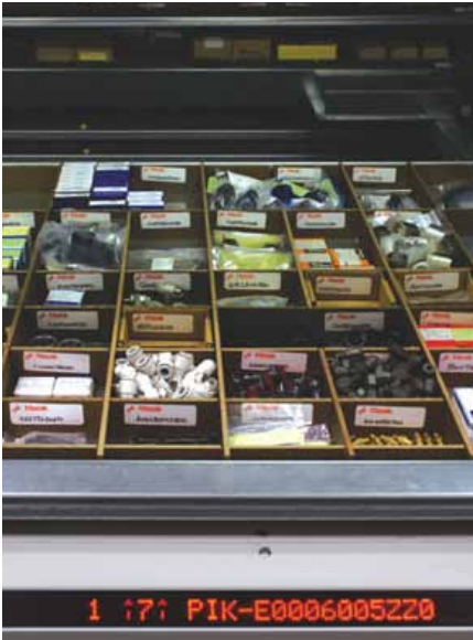
Above: The VLM automatically delivers and stores trays of parts managed by the center. Below: Operators use light-directed picking to pick parts from the trays and place them in totes.
