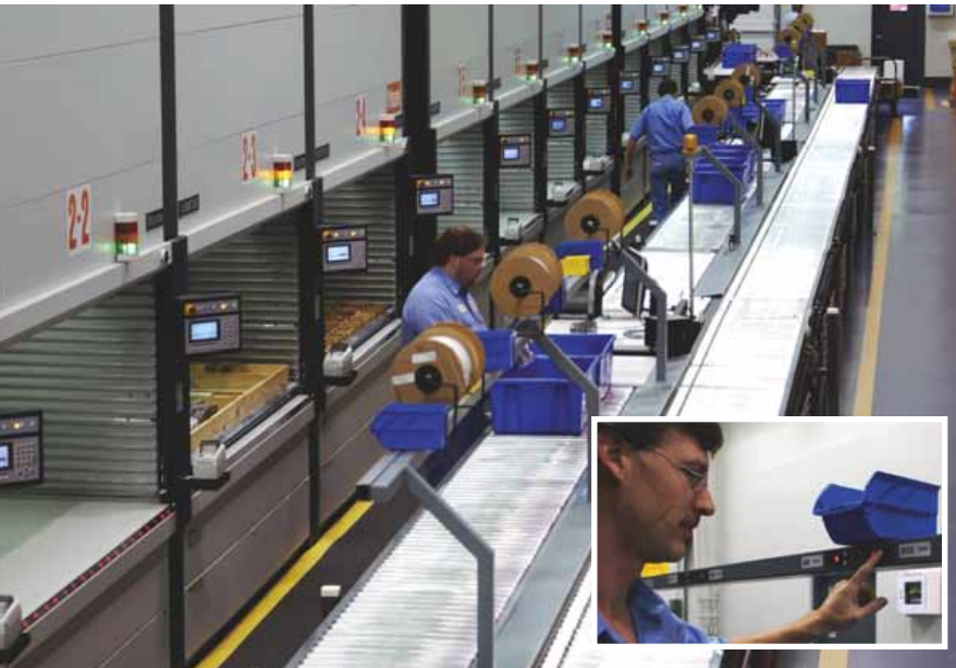
Above: The VLM automatically delivers and stores trays of parts managed by the center. Below: Operators use light-directed picking to pick parts from the trays and place them in totes.
