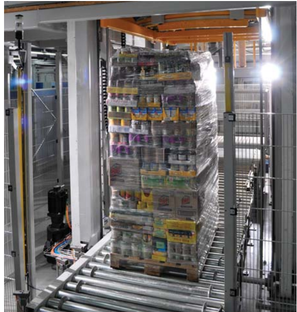
A shrink-wrapped pallet exits an automated, mixed-case palletizing system.
