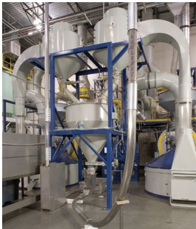
Vertical conveyors move coffee to the roaster at Apffels. photo courtesy of Cablevey
