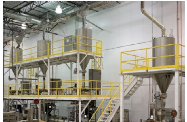
Packing bins at Apffels. Each conveying system has strengths in moving green versus ground versus whole-bean coffee. | photo courtesy of Cablevey
