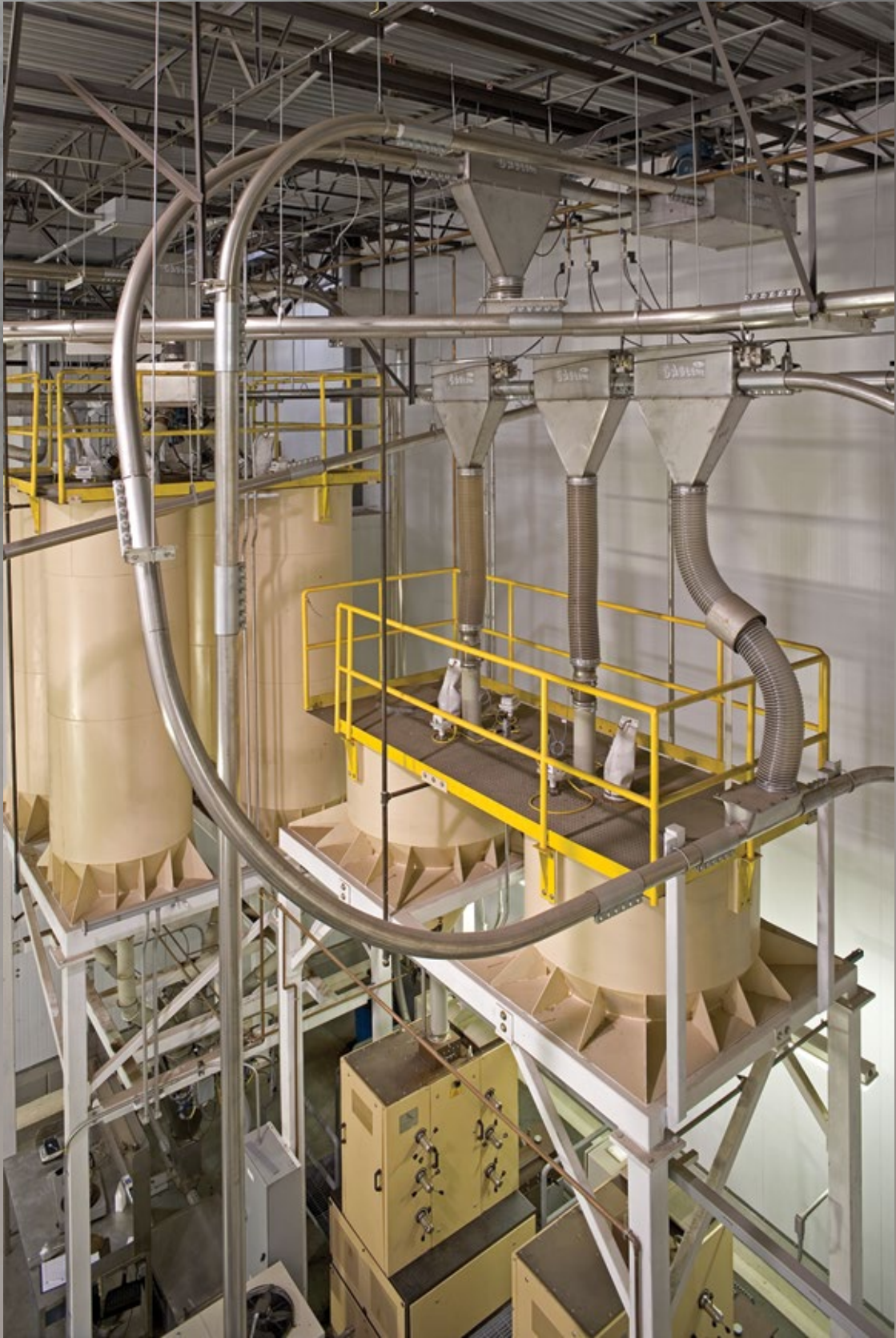
At the Apffels roasting plant, conveyors move roasted beans to grinders. | photo courtesy of Cablevey
