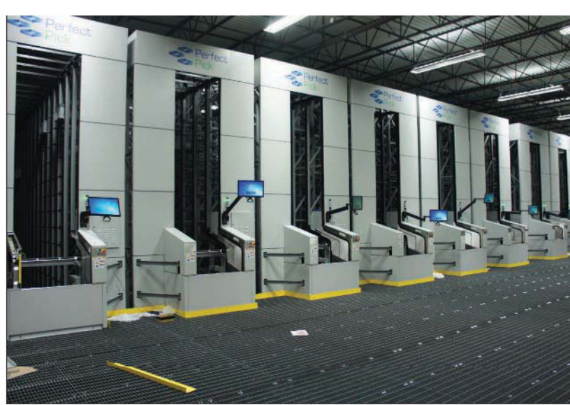
The Perfect Pick system, from the Material Handling division of OPEX Corp. ( www.OPEX.com ) exemplifies the new generation of shuttle-based picking methods.
