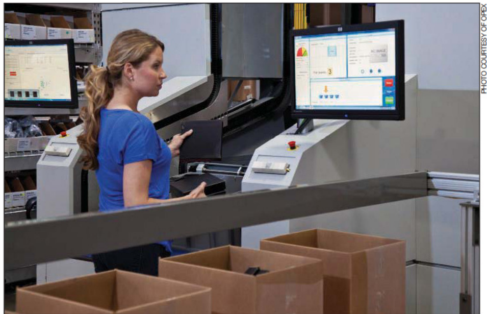
A picking monitor directs an operator to choose required items for an order and indicates where to place them.
