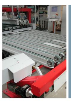
The first piece of Grenzebach equipment to exclusively utilize this advanced automation technology is the company's new High-Speed Stacker. Designed to increase glass manufacturer's efficiency and flexibility, it was developed for stacking small glass formats with high cycle times, and is currently the only device which can stack glass sheets in less than a one-second cycle.
