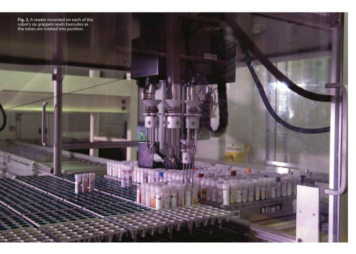
storage and retrieval system in the freezer for archiving. Likewise, specimens exiting the freezer from the automated storage and retrieval system must again be precisely positioned to accommodate the exact placement of the AutoSorter robot grippers in the refrigerator before releasing to the laboratory. This is accomplished through a specialised system of continuous-motion input and output Shuttleworth conveyors.
