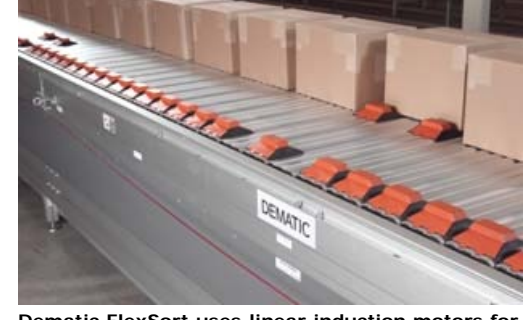
Dematic FlexSort uses linear induction motors for non-contact movement.
