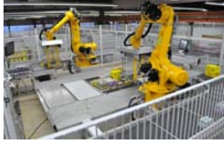
Dual robots building a pallet in AMCAP cell.
